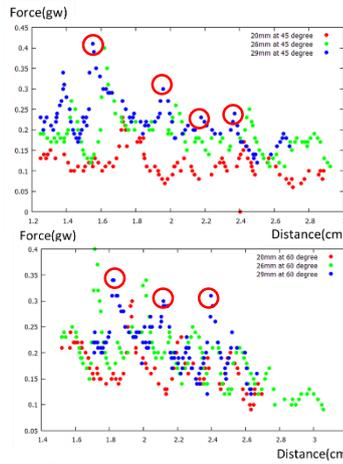
Figure 4, acoustic radiation force of 45° and 60°.
