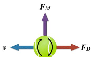
Figure 3. The schematic of backspin
