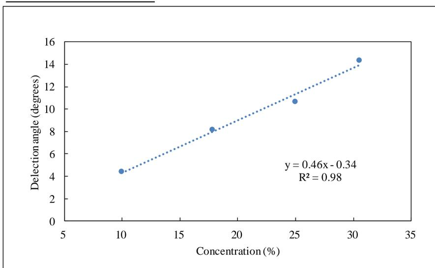
Fig. 2. The graph shows the relationship between concentration and deflection angle in 25°C.
