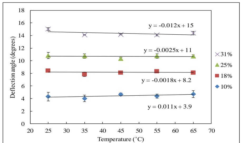
Fig. 3 The deflection angle in different concentration, depending on the temperature.
