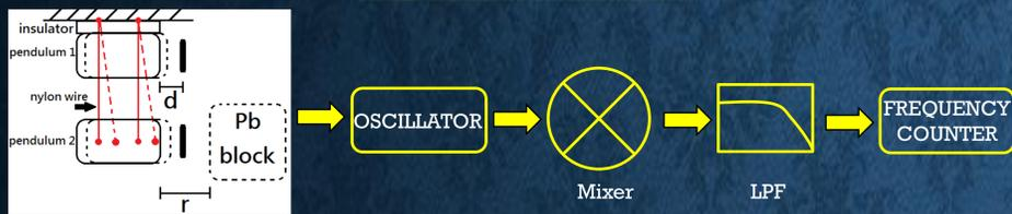
1. To cancel the effect of thermal expansion, we need two oscillators in the same condition. Thus, we set two brass cylinders and copper plates to be capacitors. The cylinder (a) was locked on the top, and the other one (b) was suspended by four nylon wires to control it only to shake forward and backward. The other side are two copper plates which were made on a printed circuit board (fig. 2).
