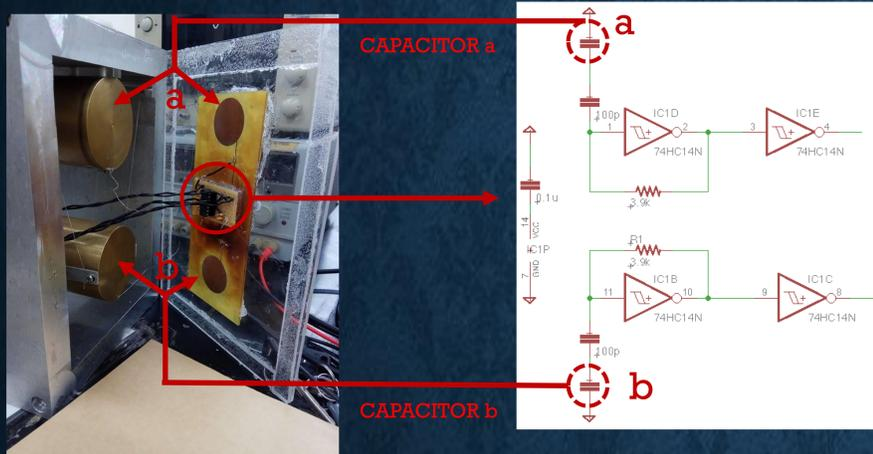
fig. 2 experiment set-up
