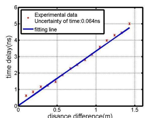
Fig. 10 : The experimental data and fitting line ( $t = (3.288 \pm 6.64 \times 10^{-2})x + 0.0112$ ) (the sampling of the oscilloscope lead to the uncertainty of the time delay.)
