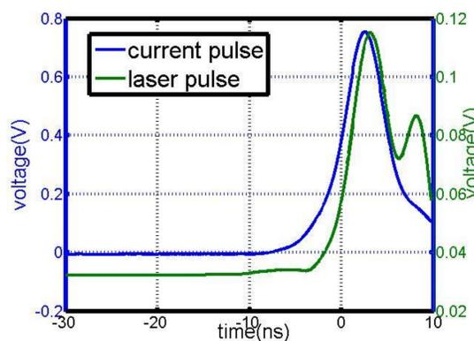
Fig. 9 : Comparison of two signals' time difference (the current pulse has 10X attenuation and laser pulse is reversed. This waveform is averaged 128 times)
