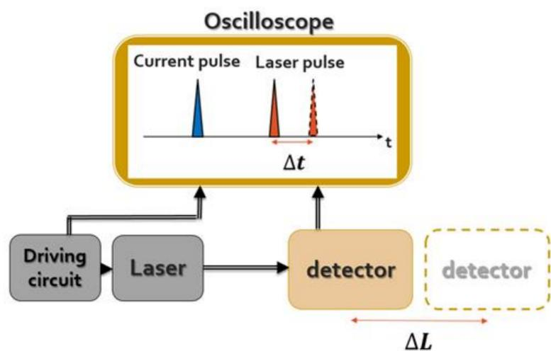
Fig.1 : Diagram of experiment set up
