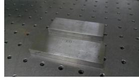
Fig. 6 : block gauge (size : 90 mm and 100mm)
