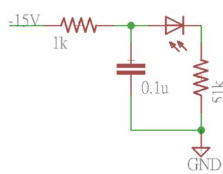
Fig.3 : Detector circuit (photodiode with reverse bias)
