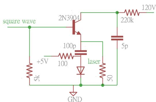
Fig.2 : The laser driving circuit (Avalanche pulse generator)
