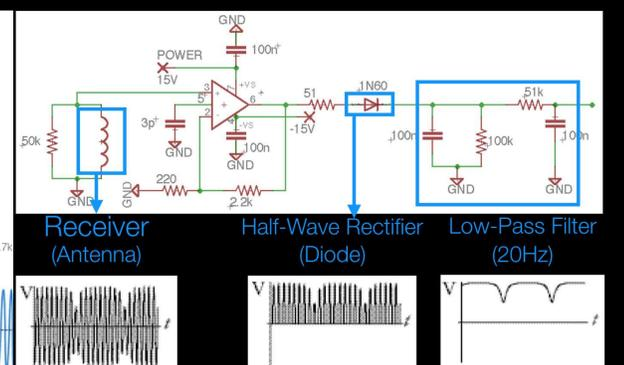
• Figure 3, Detector circuit
