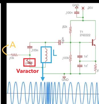
• Figure 2, Voltage controlled Oscillator
