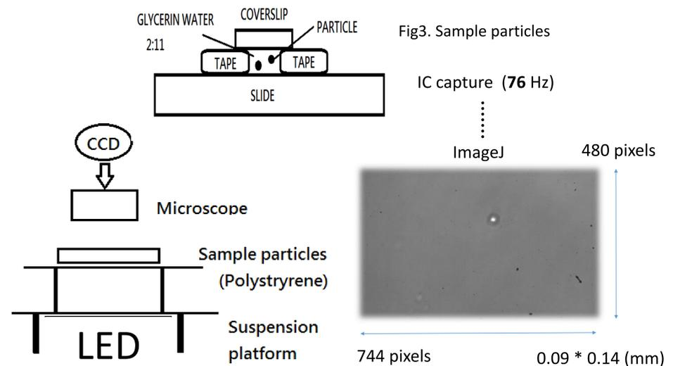
Fig4. Experiment set up
