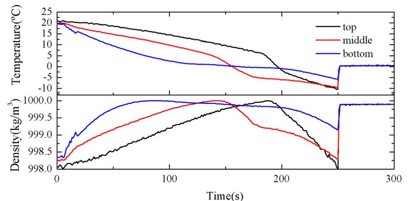
Fig. 2 temperature and density of sample water as a function of time in three different vertical position of test tube.
