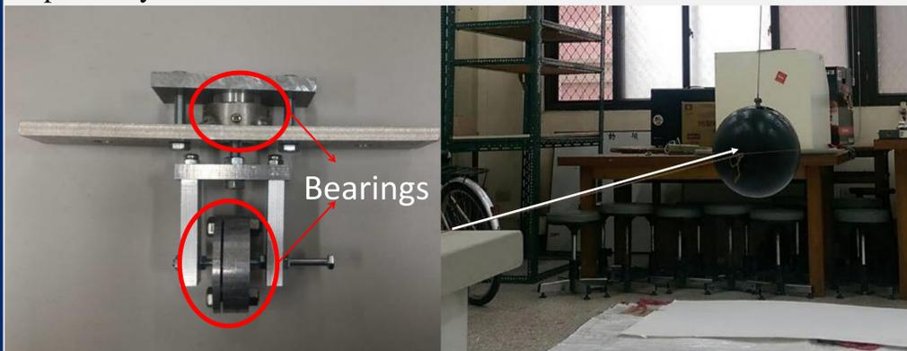
Figure 1. Pendulum support consists of Figure 2. The pendulum is tied to the table two bearings that makes the oscillation by the cotton thread (white arrow) to and rotation of the pendulum possible. setup its initial conditions.
