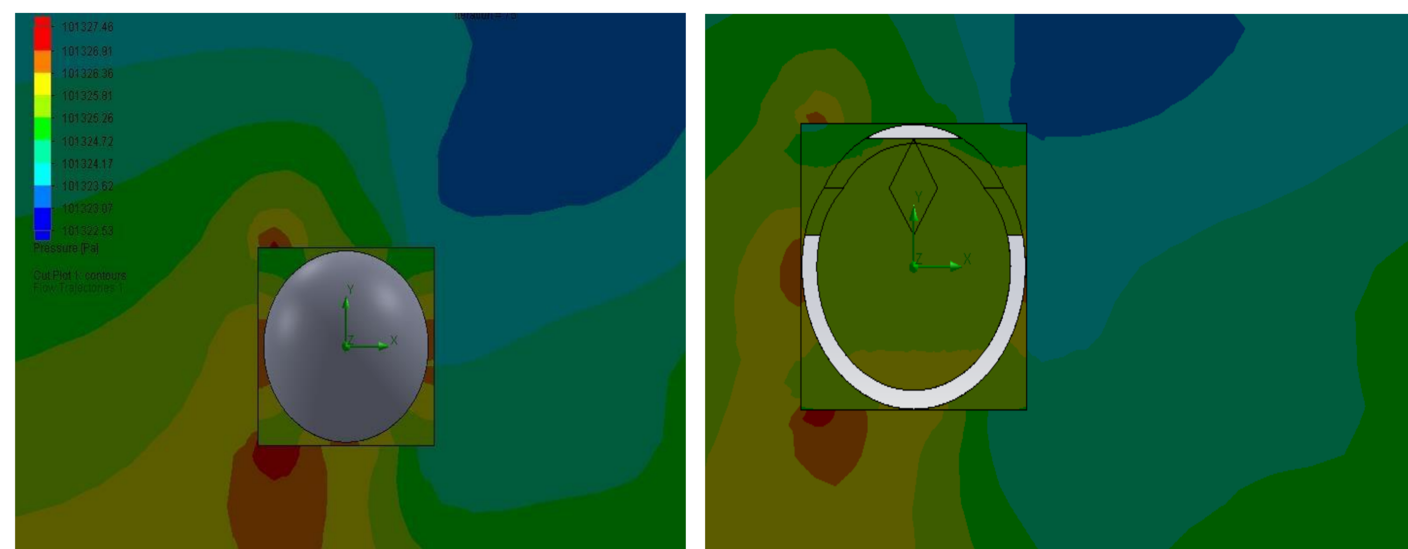
Fig 6. Intact sphere Fig 7. Four holes (With wind speed 2m/sec, rotational speed 200rpm)
