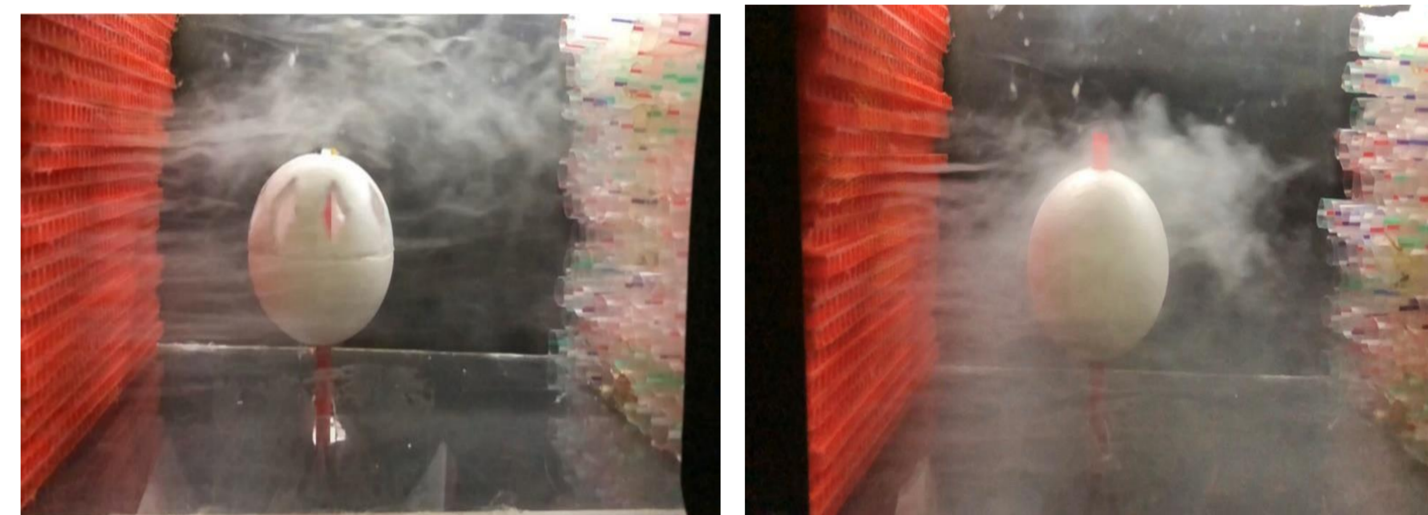
Fig 8. Flow field of ball (eight holes) Fig 9. Flow field of ball (sphere)
