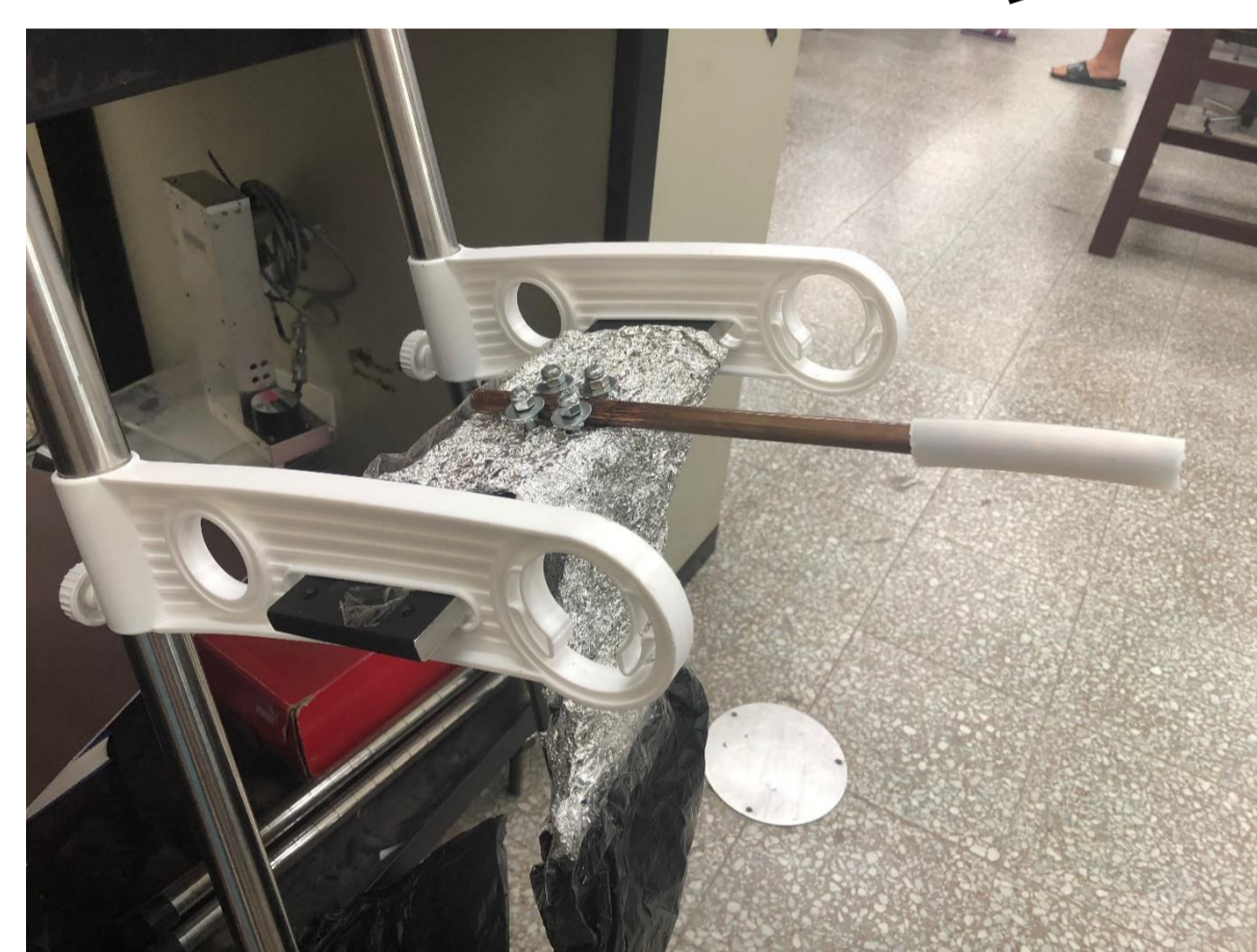
Fig.2 Holders, platform and copper core
