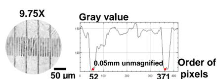
Figure 6 : Zoomed in 5.16X image of micrometer with magnification 9.75X
