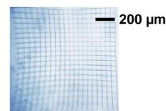
Figure 7: Image of grid with spacing 50 μm with distortion
