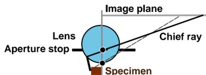
Figure 2: Pincushion distortion, larger magnification at the corner of the image, resulting from the light blocked out by the aperture stop, leading to shorter focal length.
