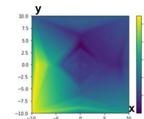
Figure 8: Distortion, different magnification throughout the field of view, is 16% on average.
