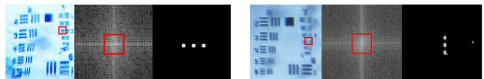
Figure 10: Best resolved pattern of element 3 in group 7 in 1951 resolution test target through lens of diameter 3 mm, with resolution 3.11 μm, analyzed from Fourier image of it.
