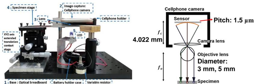
Figure 4 : Frame of single lens microscope and schematic diagram of the optical system
