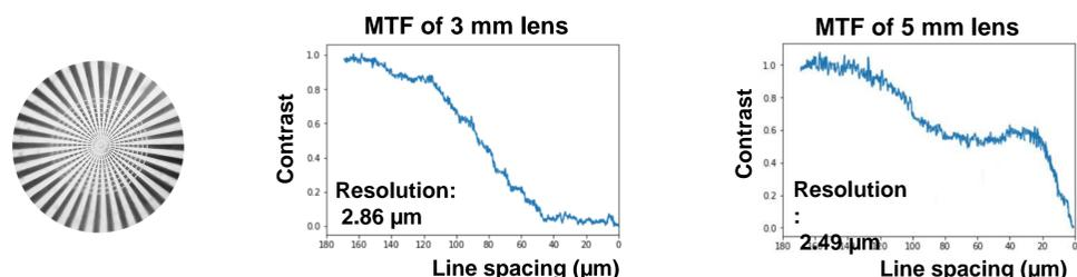
Figure 12: Figure on the left is image of Sector star applied to analyze MTF. The details of image cannot be distinguished beyond the cut-off frequency. For 3 mm lens, the closest details that can be resolved at spatial resolution 2.86 μm, and at 2.49 μm for 5 mm lens, inferring that resolution decreases with increasing diameter of lens.
