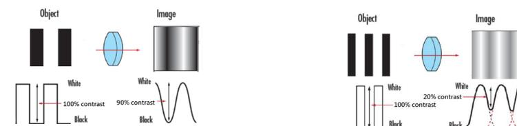
Figure 9: As spatial frequency increases, the images produced in microscopes appear as a composition of sinusoidally varying intensities that has reduced contrast, representing dark gray and light gray alternately instead.
