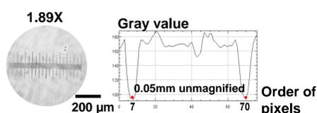
Figure 5: Image of micrometer with magnification 1.89X
