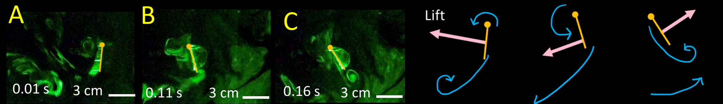
Rotational circulation (happens at A and B) is related to viscous forces. The viscous force maintains the position of the trailing edge flow, so the wing pulls the flow during rotating. The pulling force generates a reverse force on the wing.
