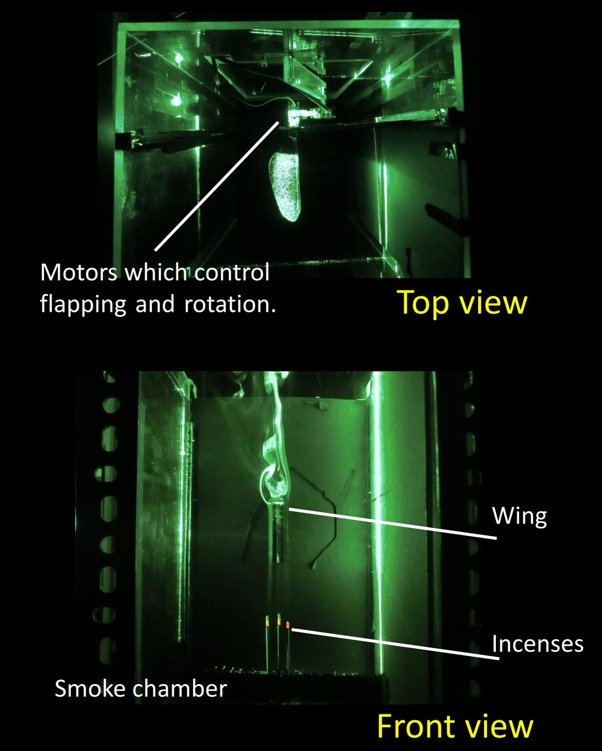
The mimic wing motion is achieved by two motors which control flapping and rotating. Incenses are put under the chamber so that the flow field can be tracked by smoke. Moreover, a laser sheet scattered by glass cylinder is useful to see two-dimensional field.
