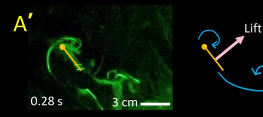
Delayed stall happens when a vortex stays at the leading edge of the wing. The flow on the wing is accelerated by the vortex. The wing is lift based on Bernoulli's law that flows with higher velocity get lower pressure, and vice versa.
