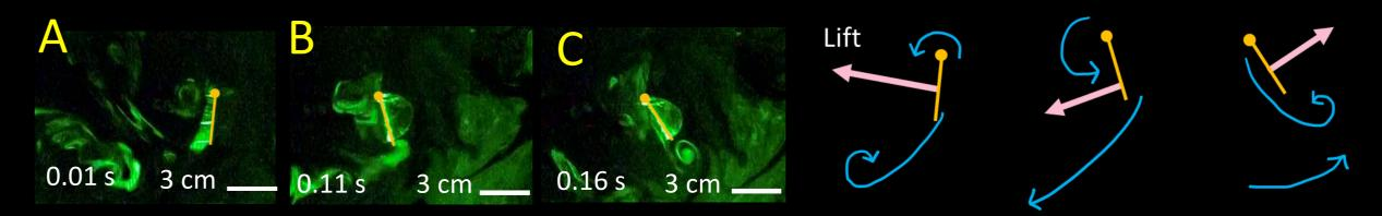
Rotational circulation (happens at A and B) is related to viscous forces. The viscous force maintains the position of the trailing edge flow, so the wing pulls the flow during rotating. The pulling force generates a reverse force on the wing.
