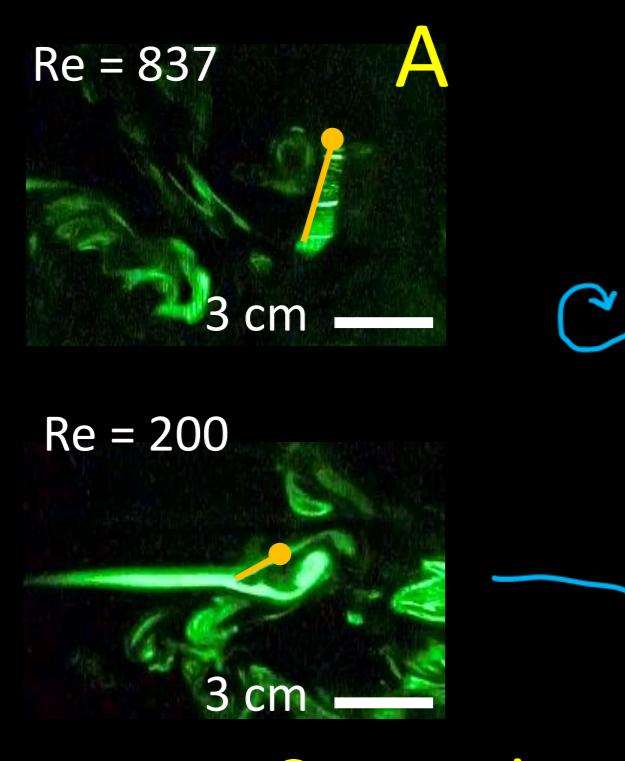
The smoke of incenses is used to be the tracker for the air flow. However, it has momentum which can destroy the vortex generated by the wing. We use less smoke in order to eliminate this effect.
