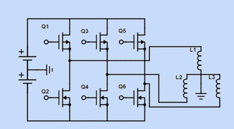
To control the motor, the ESC which is composed of six MOSFET is necessary. The positive and negative signals are sent into the coil in order with the phase of 60°.
