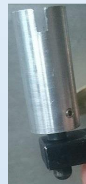
Fig.9 Fine adjustment: We use a groove to stuck the shaft of motor. So the screw and the stepper motor can be rotating synchronously.
