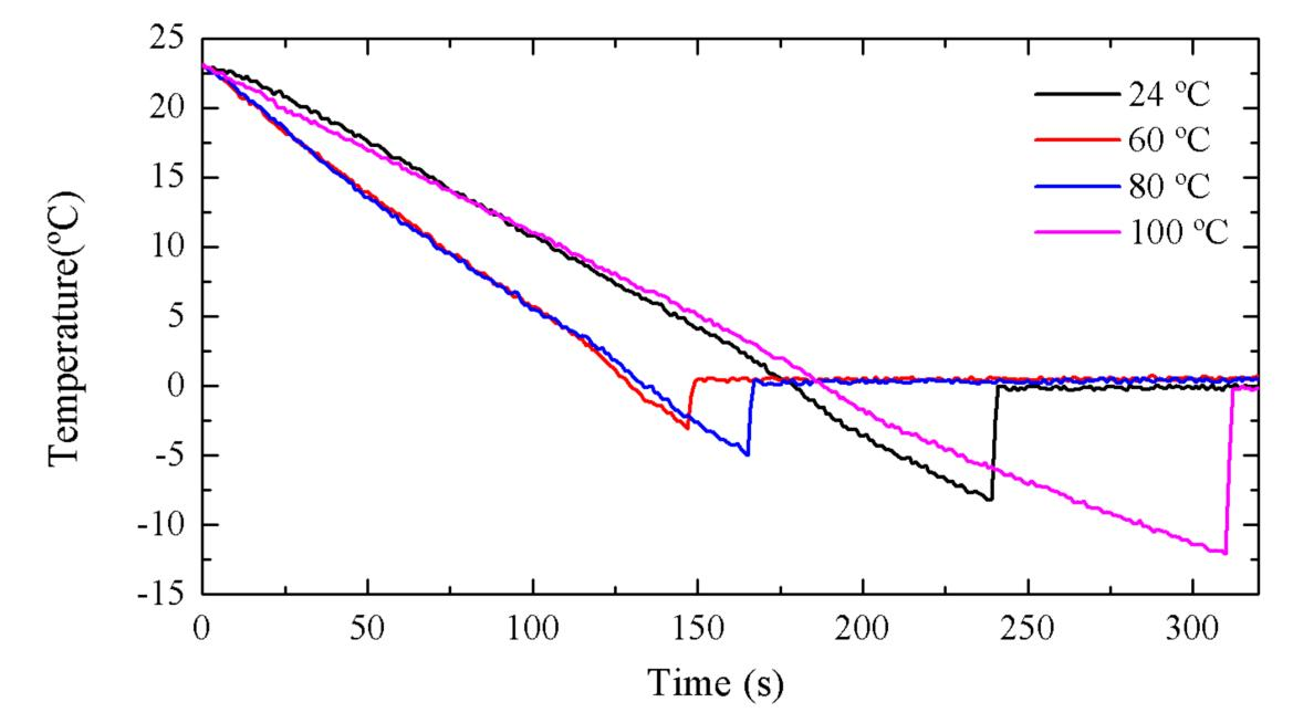
Fig. 3 The temperature as function of time of samples prepared at several different temperatures.
