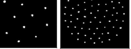
How to "trap" the charged particles? According to "Earnshaw's theorem" : it is not possible to create a static configuration of electric fields that traps the charged particle in all three directions. If we want to trap charged particles, we should produce an alternating potential. Due to all of the trapped particles with homogeneous charge, there are Coulomb repulsive force between each particle. So they will be mutually repulsive and arranged by force equilibrium, namely, "Coulomb cluster".
